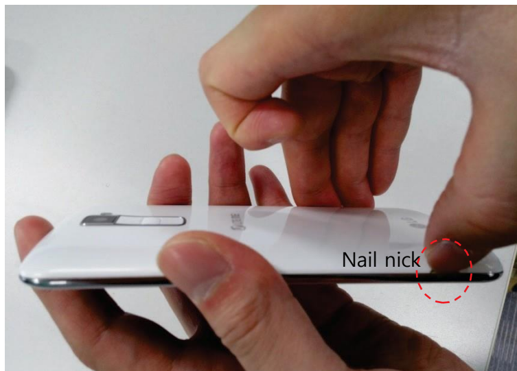
Removal of battery cover using nail nick shown in red circle
