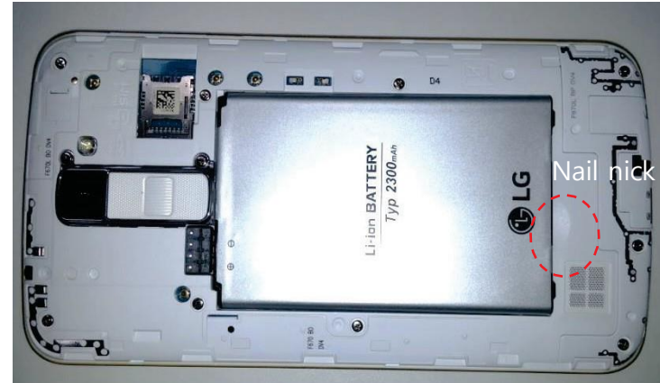
Removal of battery using nail nick shown in red circle
